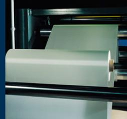
TS7 is a B-staged silicone prepreg based on a medium weave glass fabric suitable for the manufacture of tubes and laminates.
